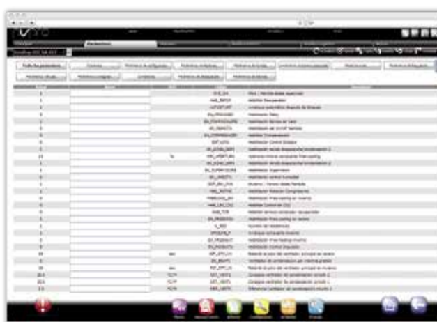
Screen with full list of settings (access according to user level): allows reading/modification of values as well as saving them (backup copy).
