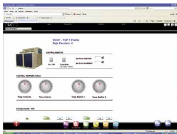
Customised screen for rooftop, basic controller of the unit: makes it possible to carry out basic operations: ON-OFF, change cooling/heating mode, change temperature setpoints and visualise the status of the main components.
